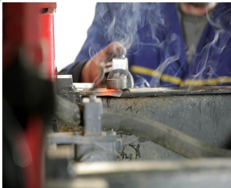
The heat is generated directly in the heart of the metal, at a depth of 5 mm. The heater brings metal to red hot temperature in a few seconds.
