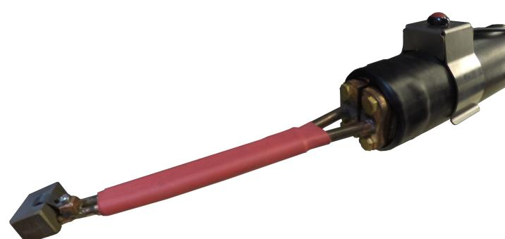
Induction enables the metal to be heated with precision in a localized spot and brings the metal up to ideal temperature.
