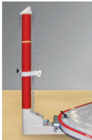
Mobile pulling tower. The tower rotates 360° around the vehicle with minimum effort.
